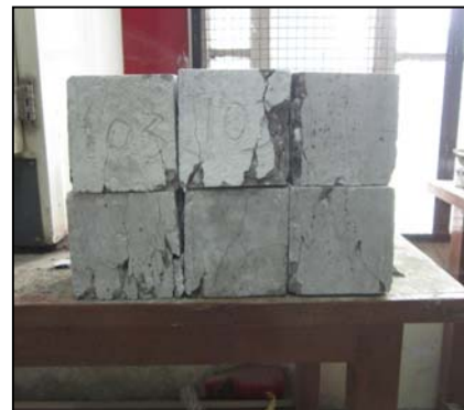
Fig.3.3: Typical Mode of Failure for Cubical Specimens.
