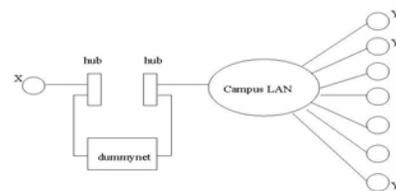
Fig. 2. Dummynet test environment
