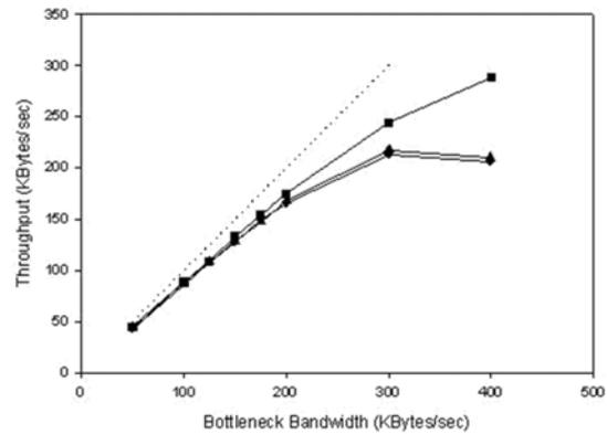
Fig. 3. TRAM performance in a network of limited bandwidth
