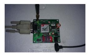
Fig: Photo of GSM Module
