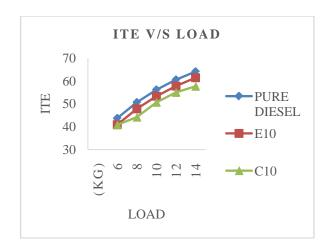
Ethanol blended fuel (E10) is closer to diesel and higher than the cotton seed oil, among the entire blend. The all blended fuel at a far cry from segment, the indicated thermal efficiency is gently increasing along with the pretty increasing load.
