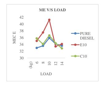
The cotton seed oil (C10) ME is also higher than the diesel but lower than the E10, among the entire blend. The all blended fuel at a far cry from segment, the mechanical efficiency is gently increasing along with load from 6kg to 10 kg after than slowly decreasing.
