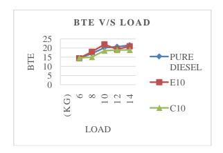
The ethanol diesel blended fuel BTE gradually increased from load 6kg to 10kg than the E10 and C10. After than it is decreased gradually. The all blended fuel at a far cry from segment, the brake thermal efficiency is gently increasing along with pretty increasing load.
