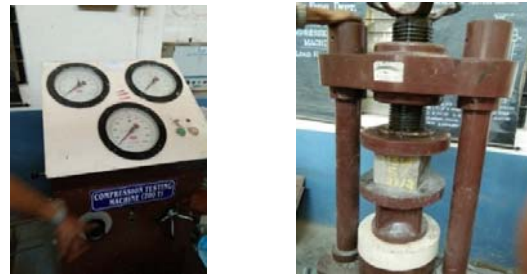
Figure 3. Compression strength test
