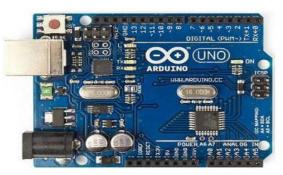
The Arduino Uno is a microcontroller board based on the ATmega328 (datasheet). It has 14 digital input/output pins (of which 6 can be used as PWM outputs), 6 analog inputs, a 16 MHz crystal oscillator, a USB connection, a power jack, an ICSP header, and a reset button. It contains everything needed to support the microcontroller; simply connect it to a computer with a USB cable or power it with a AC-to-DC adapter or battery to get started.
