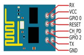
The ESP8266 is a low-cost Wi-Fi chip with full TCP/IP stack and MCU (microcontroller unit) capability. This small module allows microcontrollers to connect to a Wi-Fi network and make simple TCP/IP connections using Hayes-style commands. The ESP8285 is an ESP8266 with 1 MB of built-in flash, allowing for single-chip devices capable of connecting to Wi-Fi. The successor to these microcontroller chips is the ESP32.
