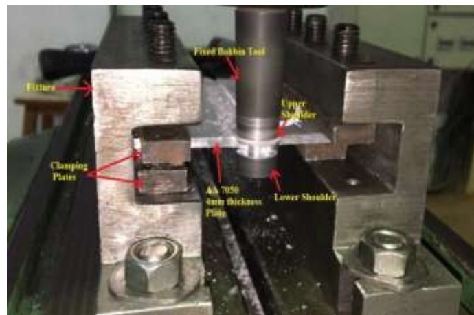
Figure5:Developed fixturewithbobbin toolweld application
