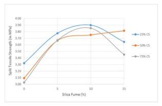
Figure 3 showing the comparison of Split Tensile strength with various percentages of Copper Slag and Silica Fume at 28 day's age of concrete
