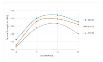
Figure 4 showing the comparison of Flexural strength with various percentages of Copper Slag and Silica Fume at 28 day's age of concrete
