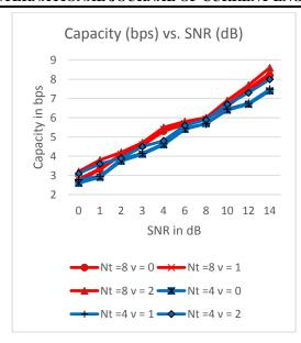
Fig 4: Channel capacity values for Nt=4 and 8 for different **v** values
