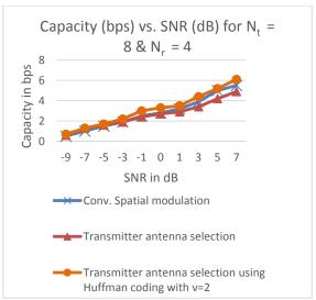
Figure 3: Performance comparison of the conventional spatial modulation scheme with adaptive scheme
