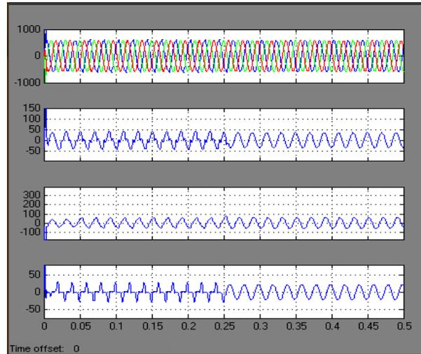
Fig 8: Source voltage and currents versus time (secs)
