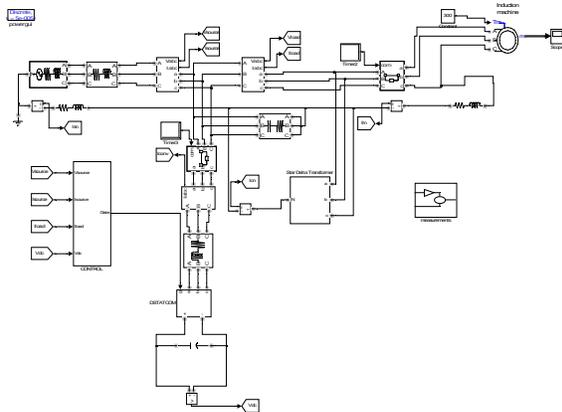
Fig 11: Simulation model with Induction Motor Load
