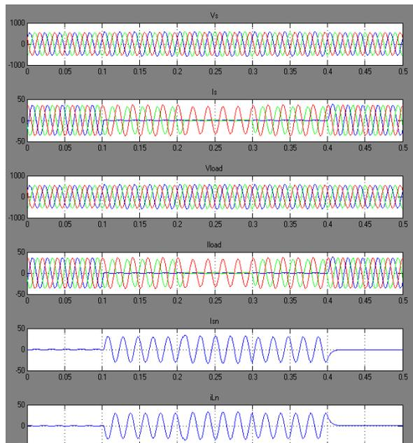
Fig 17: Source voltages and currents, Load currents versus time (secs)
