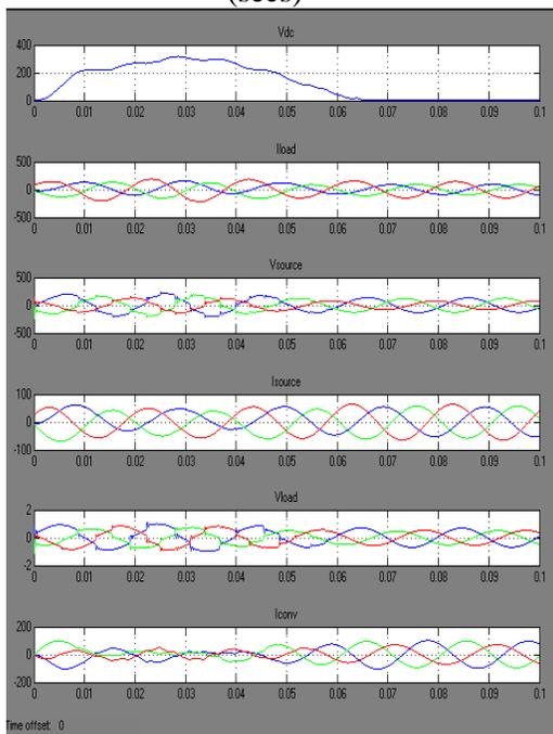
Fig 25: Source voltages and currents, Load currents versus time (secs)
