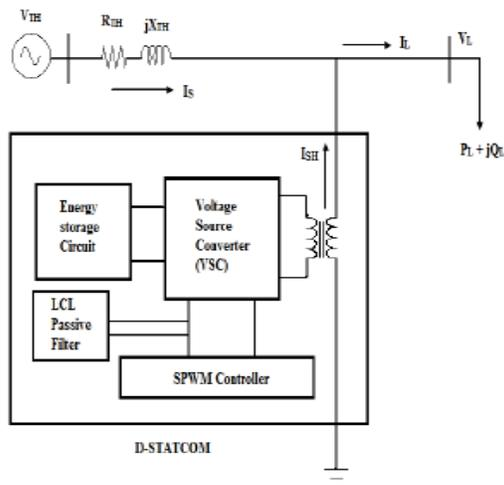
Fig 1: Schematic Diagram of D-STATCOM
