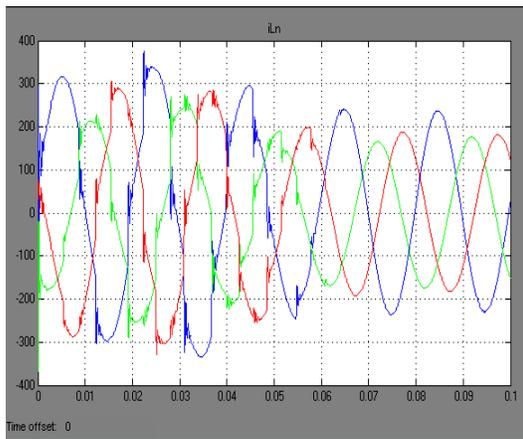
Fig 24: Neutralizing currents versus time (secs)
