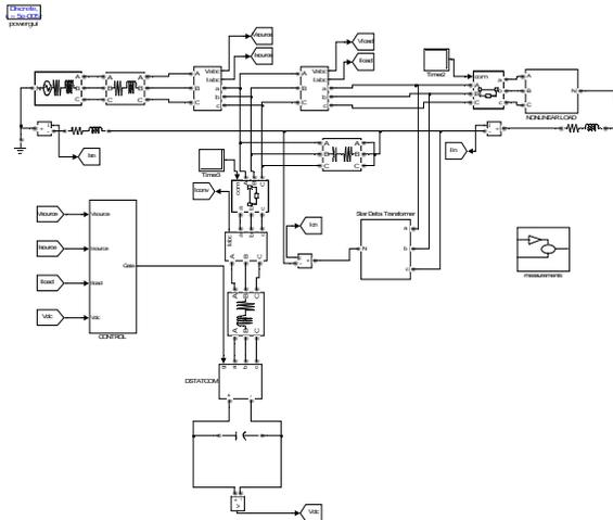
Fig 6: Simulation model with Non-Linear Load
