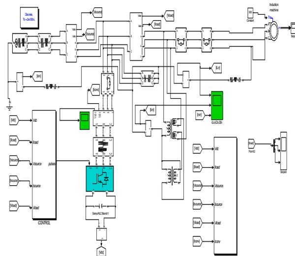
Fig 23: Simulation Model with Induction Motor
