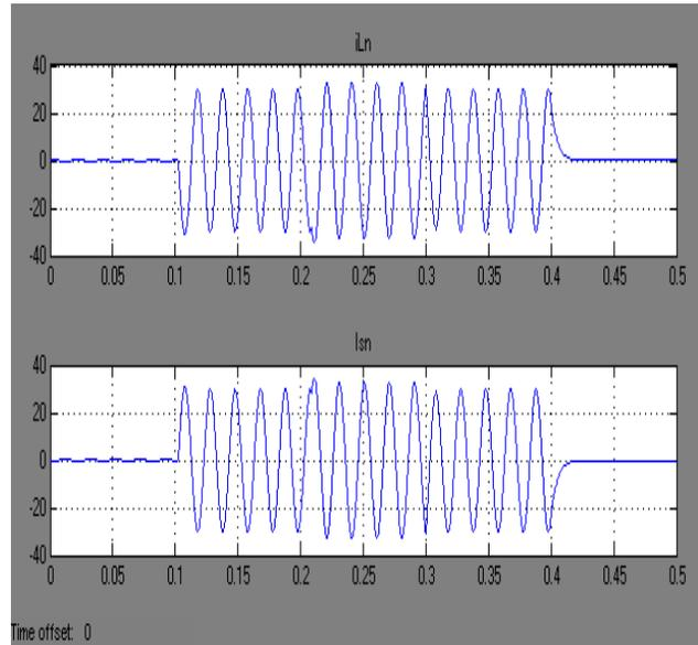
Fig 18: Neutralizing currents versus time (secs)
