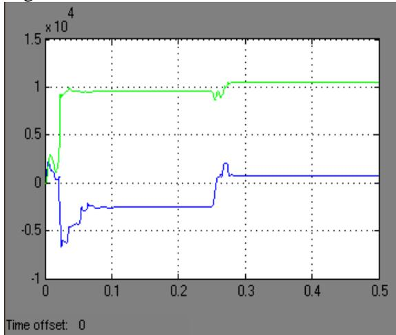
Fig 7: Active and Reactive power versus time (secs)
