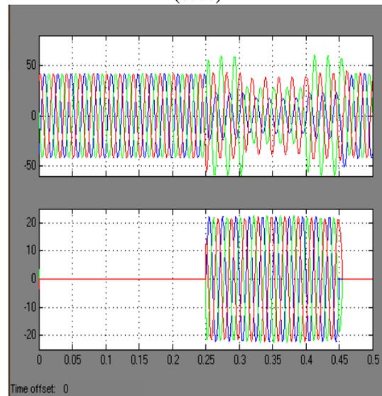
Fig 4: Source and Converter currents versus time (secs)
