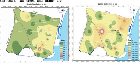
The EC values (umho/cm) of all samples were measured at  $25^{0}$ C with portable water quality kits. The conductance of surface and ground water has wide range, of course and in some areas maybe as low as 50 umho/s where precipitation is low in solutes and rocks are resistant to attack. In other areas, conductance of 50,000 umho/s or more may be reached. This is approximately conductance of seawater. The electrical conductivity is ranging from 820 – 4300u mhos/cm. above 90% of samples are
