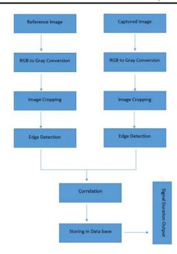
Figure 1: Block diagram representing the process of correlation and signal duration calculation
