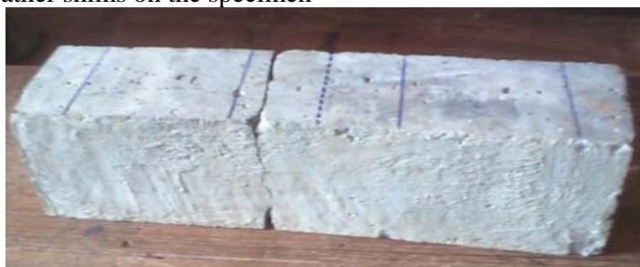
Fig: 4 Crack occurred at 1/3 rd length from support for prism
