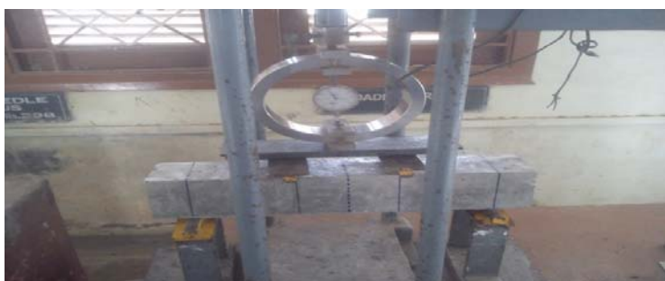
Fig: 3 Universal test setup for Flexural strength
