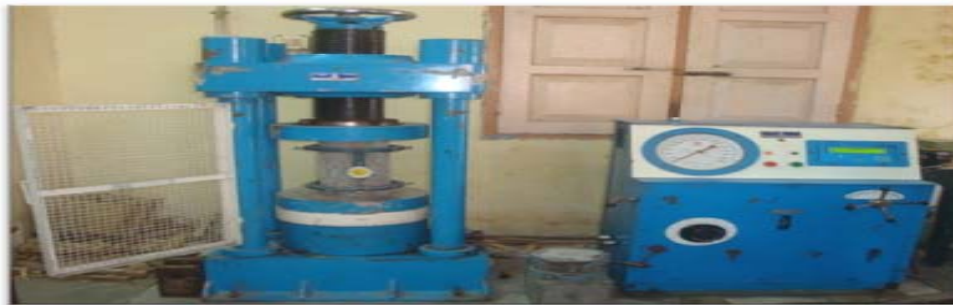
Fig: 2 Experimental setup for E – for concrete testing
