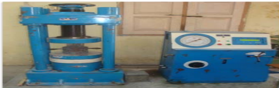
Fig 1 Experimental setup for compressive strength
