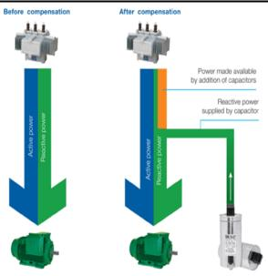
Inductance and capacitance react 180 degrees to each other. Capacitors stores KVARs and oppose the reactive energy caused by the inductor. The presence of both a capacitor and inductor in the same circuit results in the continuous alternating transfer of energy between the two. Thus, when the circuit is balanced all the energy released by the inductor is absorbed by the capacitor.
