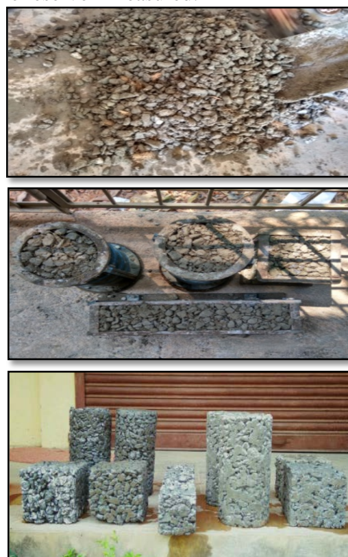
Fig 1 Preparation of CFRPC
