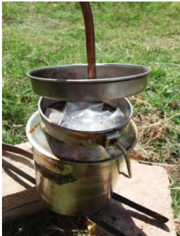
Figure 3: copper tube connected with cap of steel cane
