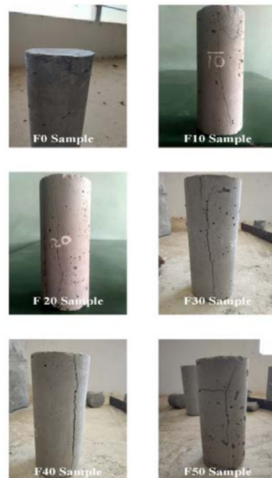
Figure 2: Failed samples in UCS Test.
