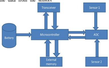
Figure 1 Block diagram of a node in agricultural WSN
