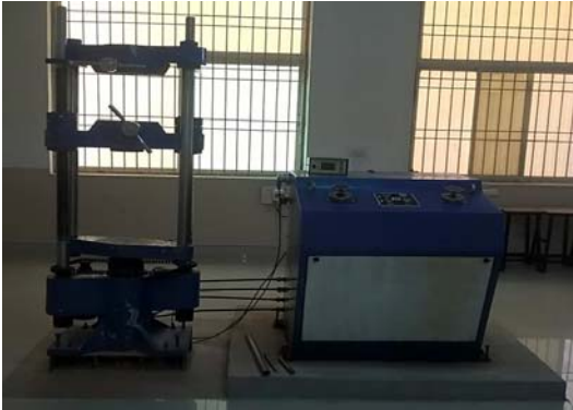
Figure 3: Experimental setup of fracture test
