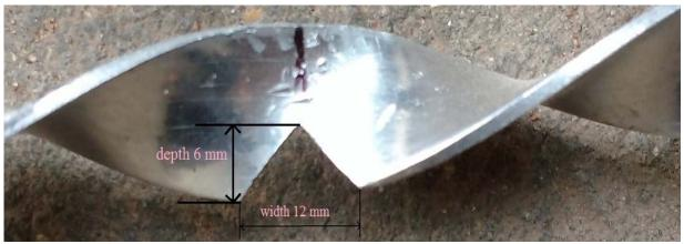
Fig.2. Photograph of v-cut twisted tape inserts
