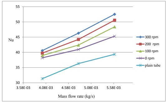
Fig. 5 Nu vs Mass flow rate
