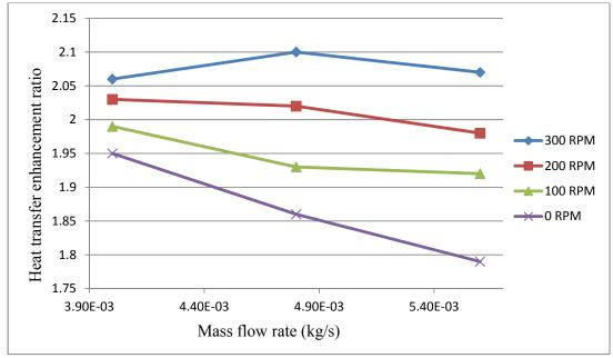
Fig. 7 Heat transfer enhancement ratio vs Mass flow rate
