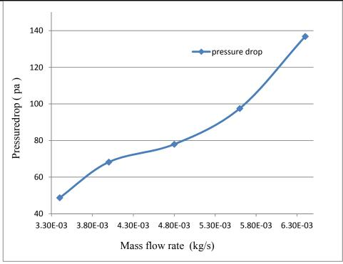
Fig.4. Pressure drop vs Mass flow rate for plain tube
