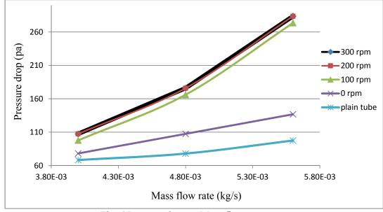
Fig. 6 Pressure drop vs Mass flow rate
