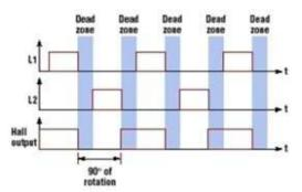
Fig. 3: Commutation Timeline Diagram
