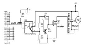
Fig.7 : PWM Generating Circuit
