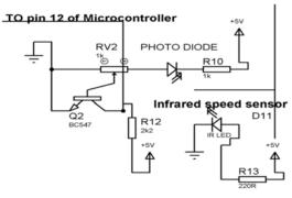
Fig.8 : Speed Sensing Circuit
