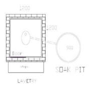
Fig. 2. Top view of Low-Cost Lavatory.
