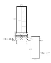
Fig. 1. Front view of Low–Cost Lavatory.
