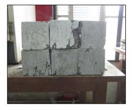
Fig.3:Typical Mode of Failure for Cubical Specimens.
