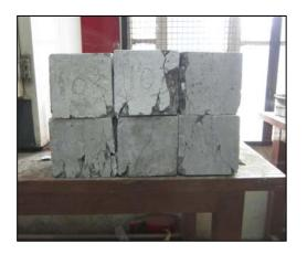
Fig.3:Typical Mode of Failure for Cubical Specimens.
